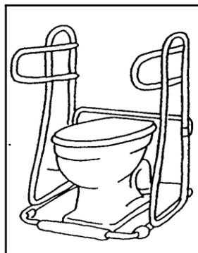
Fig. 20 Slip-over guard rails
