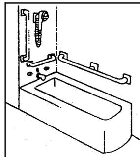
Diagonally placed grab bars (Fig. 4) are not recommended because the hand may slide and if footing is not secure, falls are more likely.
